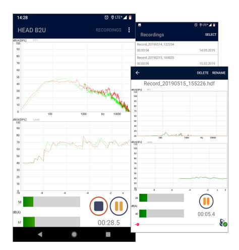
The HEAD B2U allows recordings to be started with a single tap on the recording button (image on the left). The Player displays an icon (right on the bottom of the right image) to indicate if the playback level corresponds to the recording level.
