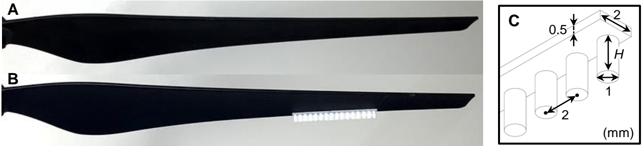
Fig. 3 (A) The basic propeller and (B) the propeller with trailing-edge attachment. (C) The dimensions of micro-structured attachment.
