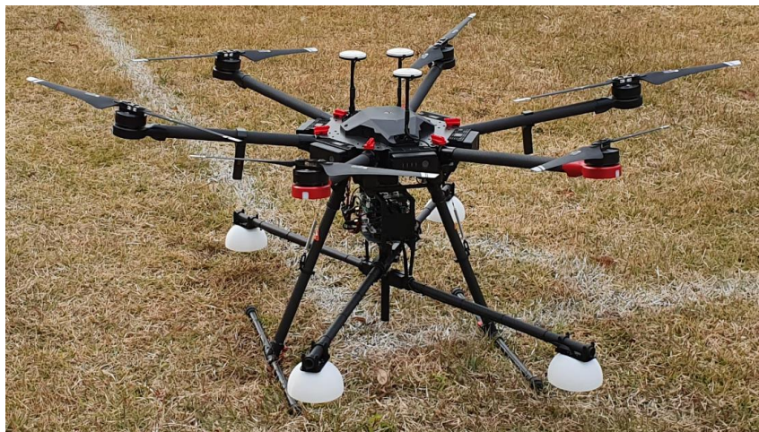
Fig. 5 32-channel microphone array system mounted on drones
