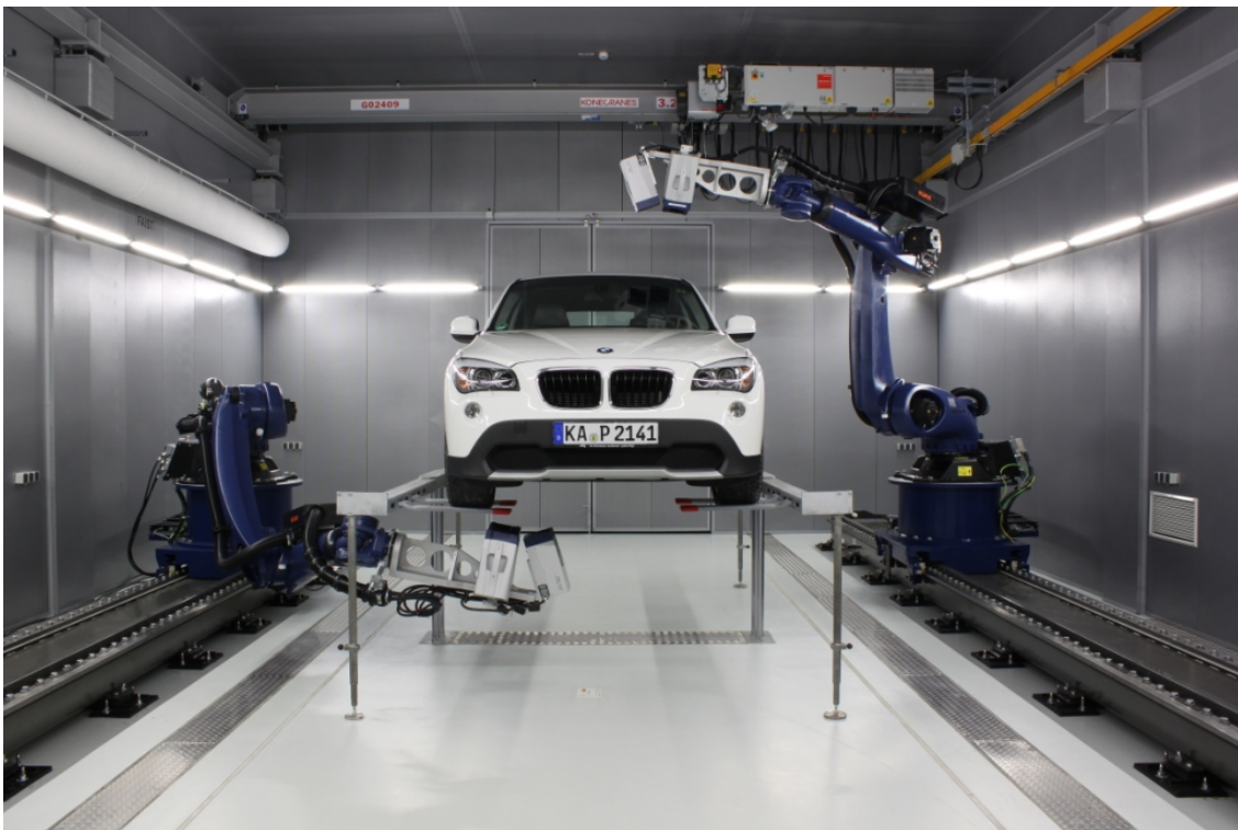
Figure 2: RoboVib test bench at Polytec GmbH in Waldbronn.
