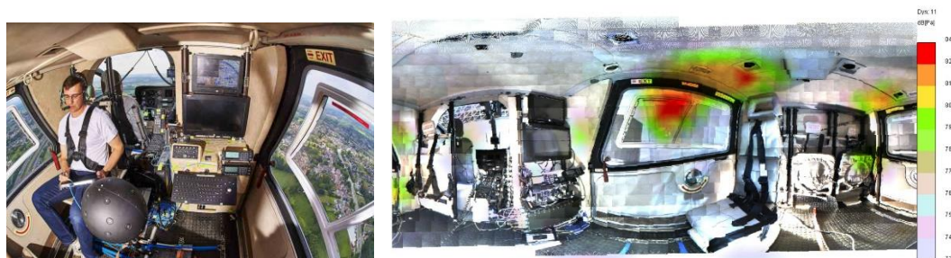
Figure 12: Spherical array allows rapid sound source localization throughout the entire aircraft cabin.
