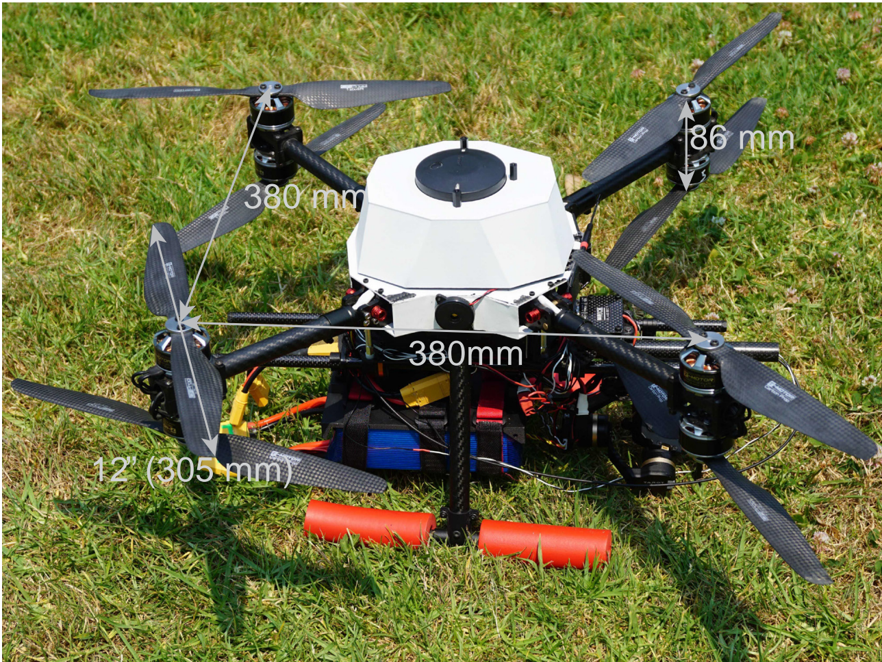
Figure 3. The custom built 4 kg quadcopter with 12"-12" propellers used for in-flight testing.
