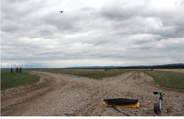
Figure 6: Audio recording in the field with a DJI S900 (left) and 200 predefined search locations quasi-uniformly distributed on a hemisphere over the array yielding an angle resolution of approximately 10^\circ (right).
