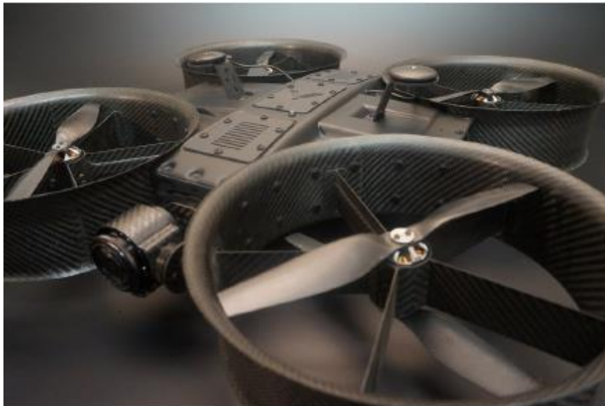
Fig. 7. Carbon-fiber duct around propeller lowers noise level of aircraft (Headrick, 2015).
