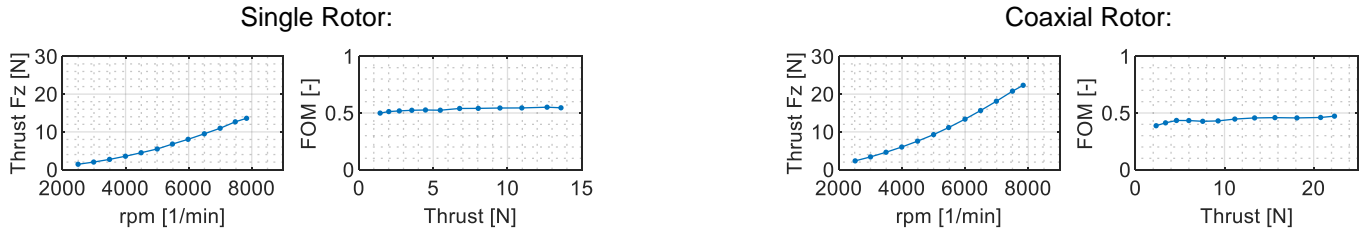
Figure 6: Thrust and efficiency (FOM) of the selected single and coaxial rotor configurations at the test-bench with X-Blades X106.
