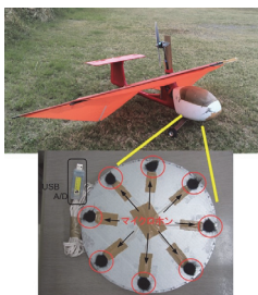
Fig. 11 Kite plane of electric motor model and its microphone array
