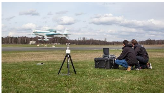
Figure 2: Impact of electric propulsion estimated with a fly-over noise measurement setup.
