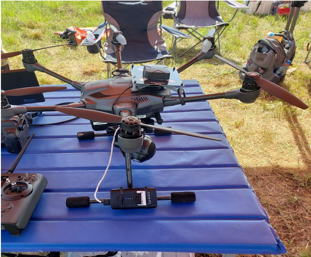
Figure 7 - Installation of Volpe miniature tracking system components on hexacopter sUAS (Volpe)
