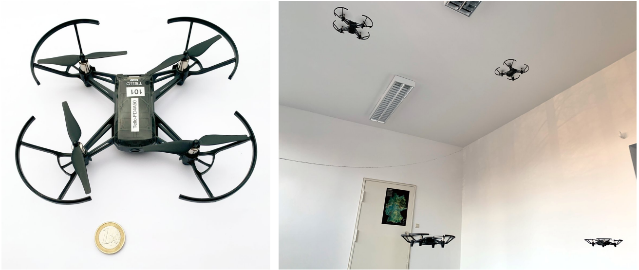
Figure 2: Tello EDU (left) and preparation of measurement flights with 4 identical Tello EDU sUAS (right)
