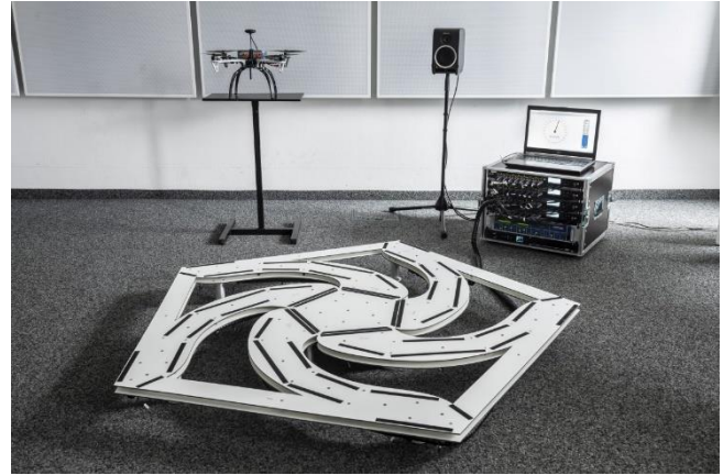
Figure 3: List of parameters (left) and picture of the 2D microphone array JR-BigSpiral31 inside the acoustic laboratory (right). The metrics BW, MSL and DI were evaluated and averaged over octave frequency bands from 125 to 16000 Hz.
