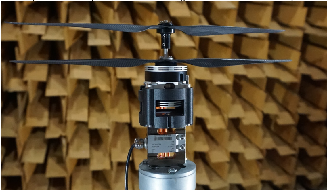
Figure 1. Contra-rotating motor unit with two 15" propellers spaced 48 mm between the hubs. The motor was mounted on a load cell in the University of Auckland's anechoic chamber.
