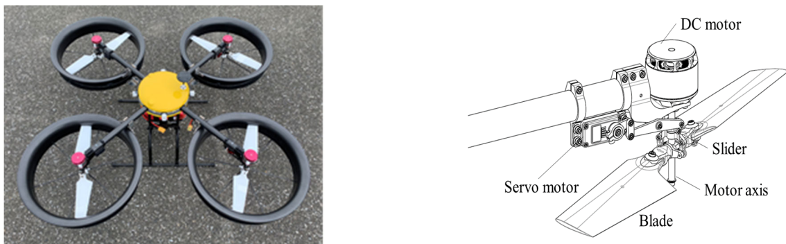
Figure 1 Quad rotor with ducted rotor (left) and variable corrective pitch mechanism
