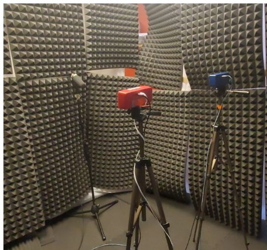
Figure 8: The setup of preliminary experiments includes a microphone, blue speaker (unaltered) and a red speaker where the polarity of the input signal is hardwired. In the PA-ANC
