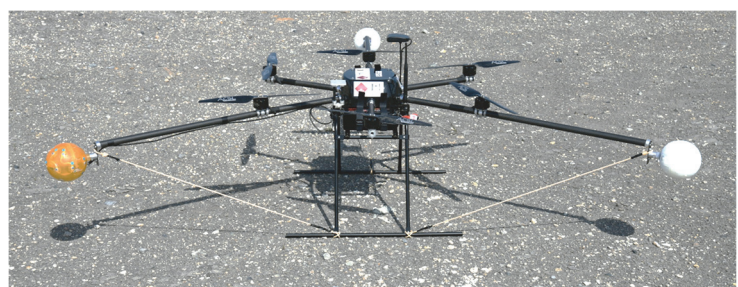
(b) 16-ch sphere microphone array coloured orange (counterweights coloured white)
